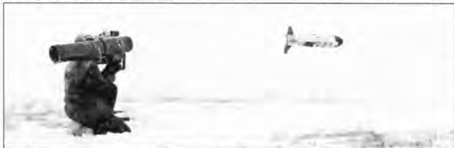
The Eryx in flight during Canadian cold weather trials: The warhead has a double charge designed to defeat reactive armour (Photo: Aerospatiale)
