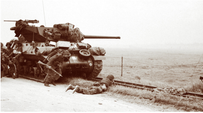
A Canadian M10 Tank Destroyer armed with a 3-inch main gun (76.2mm) and M2 50 cal machine gun.
