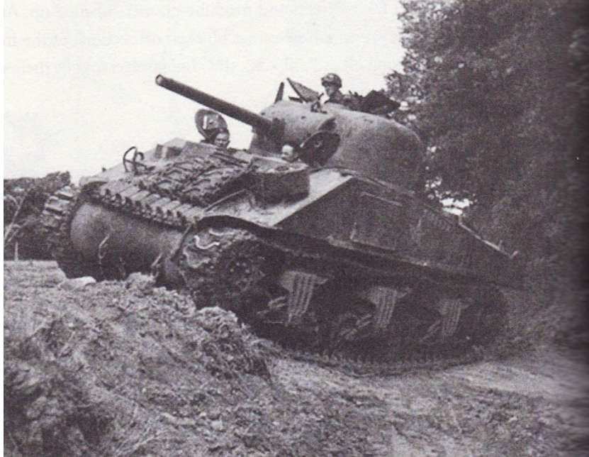
A 1 st Hussars M4A4 Medium Sherman tank with a short barrel 75mm main gun and two 30 caliber machineguns, extra track pads were often welded to the frontal armour to provide more protection.
