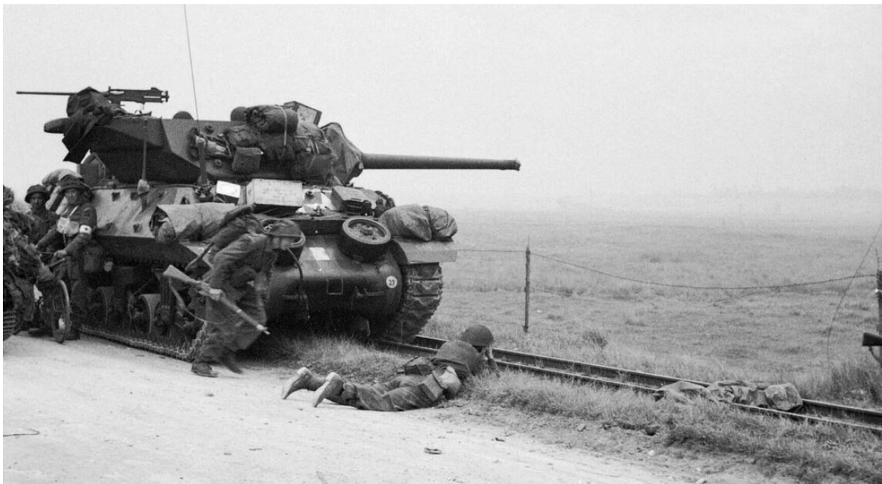
An Canadian M10 Tank Destroyer armed with a 3 inch main gun (76.2mm) and M2 50 cal machinegun.
